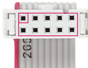
Figure 7-3: Use entire IDC10 connector for multiplexing feature
